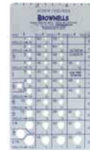
Identifies Threads Plus Gives Drill & Tap Sizes
